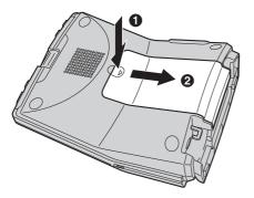
**2** Replace the old battery with a new one. Close the cover.
